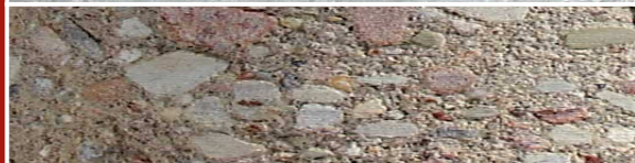
Chudy beton, f_c = 6 - 9 MPa, 20cm
